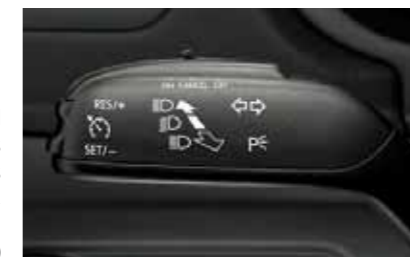
Cruise control for all engine versions (5J1 035 623 for cars without on-board computer, 5J1 035 623A for cars with on-board computer)
