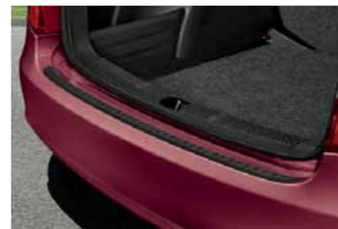
Protective cover of the rear bumper for Fabia (KDA 710 001), for Fabia Combi (KDA 720 001)
